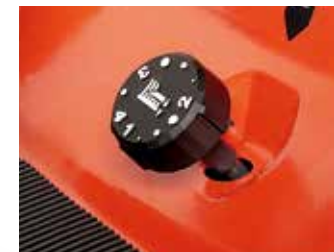
Easy reach cutting height adjustment dial
