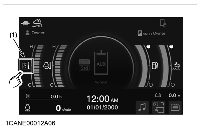
(1) Hydraulic oil temperature indicator
