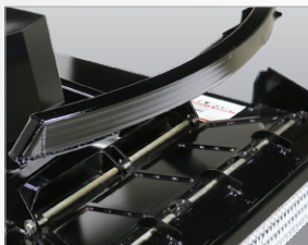
Push bar forces trees away from the operator.
