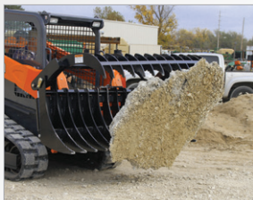
Dual hydraulic cylinders allow upper jaw to grip the material better.
