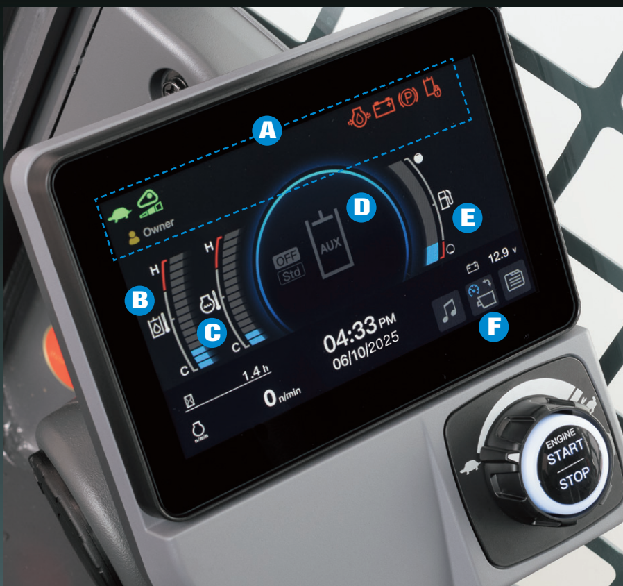
A. Situation Indicator (such as working function, battery charge indicator etc..) B. Hydraulic Oil Temperature C. Coolant Temperature D. AUX Mode E. Fuel Level F. Menu Icons
