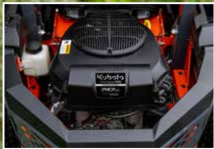
Z242KH/Z252KH model (Powered by KOHLER® 7000 Series) 22.0HP/26.0HP
